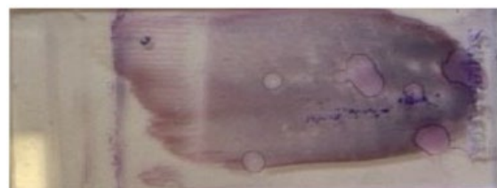
Faded smear at wrong end of slide (top), condensation damage (bottom)
